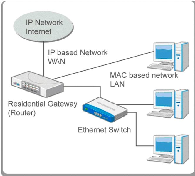
A router provides basic functions such as:
